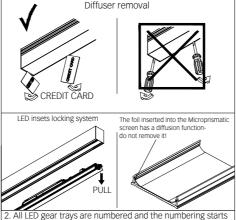
All LED gear trays are numbered and the numbering starts from the cable entry side. In non-standard luminaires the numbering of LED gear trays is made in accordance with technical drawings.
