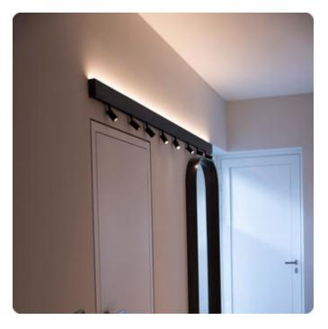
7700lm. 93W. 6,9kg. Binning initial <= MacAdam 3. IP20. Protection class I. CE, UKCA marking. Prüfzeichen: ENEC. IK02. 220-240V. 50-60 Hz. RG0 (EN62471). Luminous flux reduction up to 0,4%/1.000 operating hours. Nominal failure rate: 0,2%/1.000 operating hours. L80B10 (tq 25°C) = 50.000h. 5 years warranty. Manufacturer: Lightnet GmbH, ISO 9001:2015 and 50001:2018 certified.
