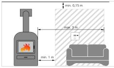
Fig. 3: Position in rooms with combustion equipment
