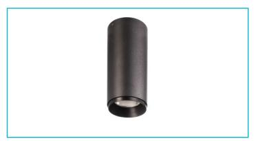
Ceiling lights in the LUCEA series are available with or without mount in the 10, 15, 20 and 30 watt output levels. The variants with mount can also be rotated and swivelled. They provide up to 2,900 lumens of light output depending on the design. The light emission angle can be narrowed or expanded by exchanging optionally available lenses.
