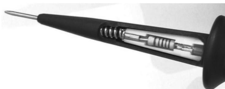
The instrument provides a high level of safety by means of two series resistors immediately behind the test electrodes as well as two absolutely independently working test systems.
