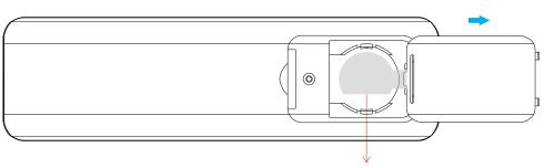
Note:Before the first use, please remove the protective film on the battery.
