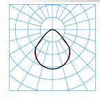
Opendo D2-L PW19 47-840 ETDD +LLWRM 01 TX277481 UGR I = 18.7 UGR q = 19.1 DIN 5040: A50 UTE: 1,00 C CEN Flux Code: 62 90 98 100 100 0 0 50 0
