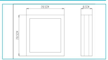
High-quality material and classic design - The Scuti series embodies the elegant fusion of brushed stainless steel and robust plastic. It features two E27 holders and therefore provides plenty of scope when it comes to choosing lamps. We recommend 2 x 6-watt LED lamps for a beautifully uniform and glare-free light pattern.
