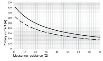
$\begin{array}{l} ---- U_{C} = \pm 15 \ V \ -5 \ \%, \ T_{A} = 85 \ ^{\circ}\text{C} \\ --- V_{C} = \pm 12 \ V \ -5 \ \%, \ T_{A} = 85 \ ^{\circ}\text{C} \\ \\ \text{Primary currents higher than } I_{PM} \ \text{only for peak!} \end{array}$
