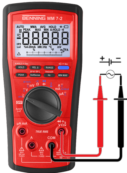
Figure 9: Voltage, frequency or duty cycle measurement
