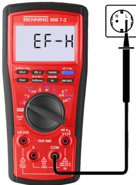
Figure 15: External conductor or phase testing
