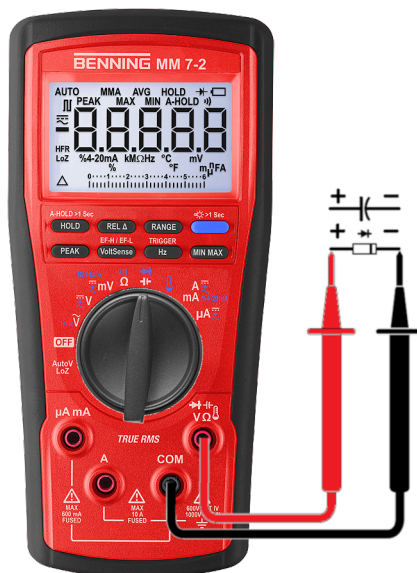
Figure 12: Capacitance measurement or diode testing
