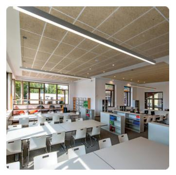
Matching luminaire's surface colour. High-power current. 3600lm. 31W. 3,5kg. Binning initial <= MacAdam 3. IP20. Protection class I. CE, UKCA marking. Prüfzeichen: ENEC. IK02. 220-240V. 50-60 Hz. RG0 (EN62471). Luminous flux reduction up to 0,4%/1.000 operating hours. Nominal failure rate: 0,2%/1.000 operating hours. L80B10 (tq 25°C) = 50.000h. 5 years warranty. Manufacturer: Lightnet GmbH, ISO 9001:2015 and 50001:2018 certified.
