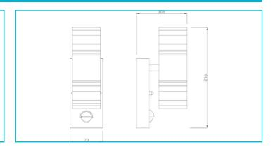
Compact, subtle, impactful - Zilly series surface-mounted wall lights can be installed on patios, building walls or in entrances to living spaces and look exquisite in any location with their stainless steel housing and light emanating upwards and/or downwards. The dimmable light sources each with max. 35 W are in GU10 holders. They are available in variants with or without movement sensors
