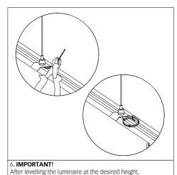
cut off the excess of the suspension cord or roll it up and secure it to avoid a short-circuit caused by contact with the light sources.
