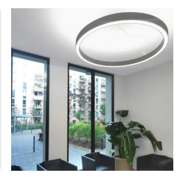
Power supply: transparent. Ceiling rose: Matching luminaire`s surface colour. Medium-power current. 19560lm. 175W. 15,9kg. Binning initial <= MacAdam 3. IP20. Protection class I. CE, UKCA marking. IK02. 220-240V. 50-60 Hz. RG0 (EN62471). Luminous flux reduction up to 0,3%/1.000 operating hours. Nominal failure rate: 0,2%/1.000 operating hours. L85B10 (tq 25°C) = 50.000h. 5 years warranty. Manufacturer: Lightnet GmbH, ISO 9001:2015 and 50001:2018 certified.
