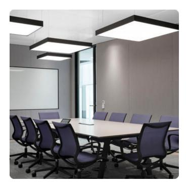
rose: Matching luminaire's surface colour. High-power current. 12379lm. 129W. 16,2kg. Binning initial <= MacAdam 3. IP20. Protection class I. CE, UKCA marking. Prüfzeichen: ENEC. IK02. 220-240V. 50-60 Hz. RG0 (EN62471). Luminous flux reduction up to 0,4%/1.000 operating hours. Nominal failure rate: 0,2%/1.000 operating hours. L80B10 (tq 25°C) = 50.000h. 5 years warranty. Manufacturer: Lightnet GmbH, ISO 9001:2015 and 50001:2018 certified.
