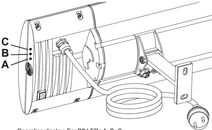
Operating display: For D2 LEDs A, B, C
