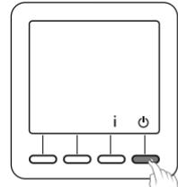
In this mode, heating is shut down.
