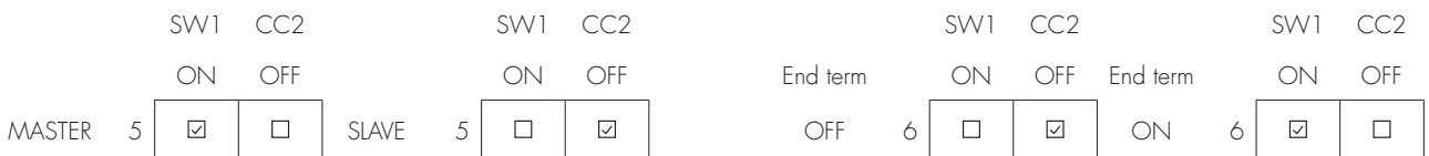
Settings explanation of Dip 5, 6 on SW1 CC2
