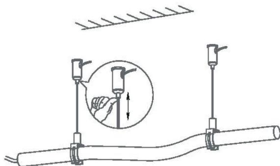
**EN:** The length of the suspension rope is adjustable when pressing the sleeve, as shown.
