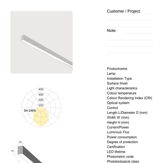
Matric-A3 LED Surface mounted light-line Silver Anodised Direct light distribution 4000K CRI>80 Opal diffuser Switchable L=2055mm W=55mm H=75mm Medium-Power 4430lm 38W IP20 Prüfzeichen: ENEC L85B10 (tq 25°C) = 50.000h 840/339 RG0 (EN62471) Indoor: ta [ambient] max. 25°C 5,2kg
