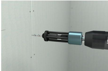
Insert the centering drill into the holder.
