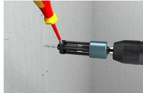
Fix the centering drill with fixing screw on the side.
