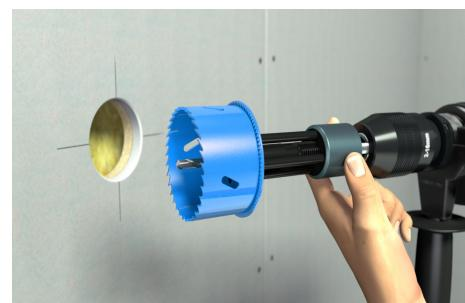
Hold the aluminum sleeve and return the adapter to the starting position by turning the drill clockwise.
