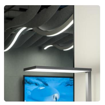
900mm. W=200mm. H=2000/25mm. High-power current. 14960lm. 114W. 20,1kg. Binning initial <= MacAdam 3. Uformed floor base matching luminaire's outer surface colour. Plug Schuko CEE 7/7 (Type E+F). IP20. Protection class I. CE, UKCA marking. IK02. 220-240V. 50-60 Hz. Luminous flux reduction up to 0,4%/1.000 operating hours. Nominal failure rate: 0,2%/1.000 operating hours. L80B10 (tq 25°C) = 50.000h. 5 years warranty. Manufacturer: Lightnet GmbH, ISO 9001:2015 and 50001:2018 certified.
